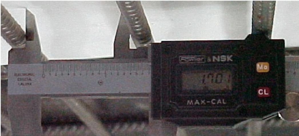
Calculate the area of the wire by using the information you received from your measurements. As example: if the diameter  $D$  is 0.126 inch: then the area is  $D \times D \times 3.1416/4 = .126 \times .126 \times .7854 = .012$  sq inch.
