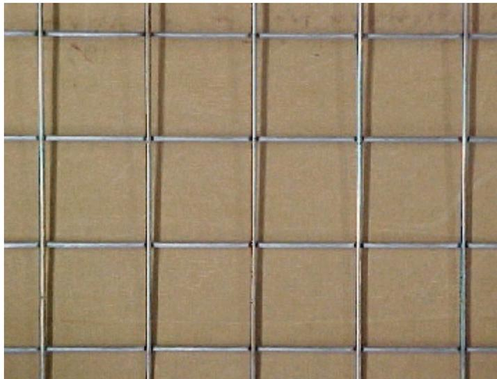
An example for a diameter of a wire could be 4 x 12 - W 2 x W 4, which means the wire W2 wire is spaced every 4 inches and the W4 wire is spaced every 12 inches.
