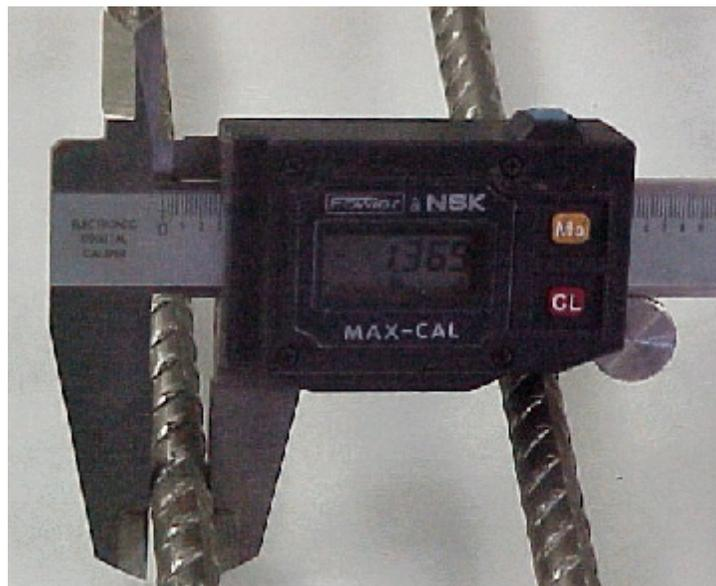
Measure the spacing between the horizontal and vertical wires.
